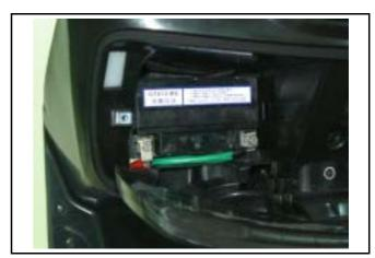
Remove the luggage box. Disconnect the cable positive terminal from the start relay.
