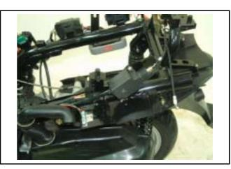
Remove the power coupler of auto by-starter. Remove the spark plug cap.
