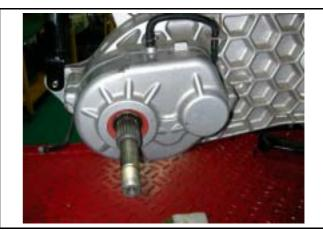
Remove final gear. Remove counter shaft, gear and 2 washers. Remove final shaft.
