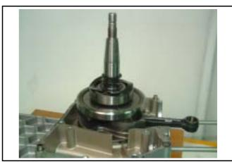
Install 2 dowel pins and new gasket.
