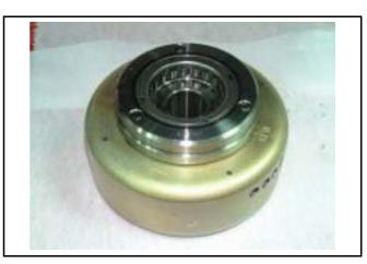
Install starting clutch driven gear onto one way clutch.
