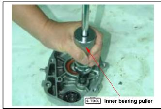
Remove oil seal, and then remove final shaft bearing from gear box cover using following tools. **Special tool:**
