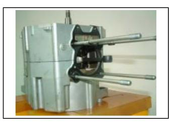
Tighten 8 bolts on the left crankcase. Tighten 2 bolts on the left crankcase. **Torque value: 0.8~1.2kgf-m**
