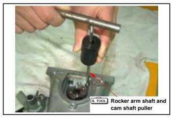
Remove cam shafts. **Special Service Tool:** Rocker arm and cam shaft puller SYM-1445100
