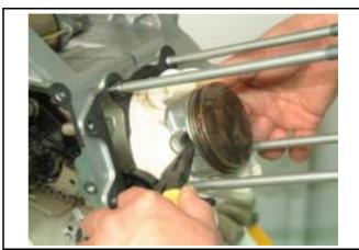
Remove cylinder gasket and dowel pin. Clean up all residues or foreign materials from the two matching surfaces of cylinder and crankcase.
