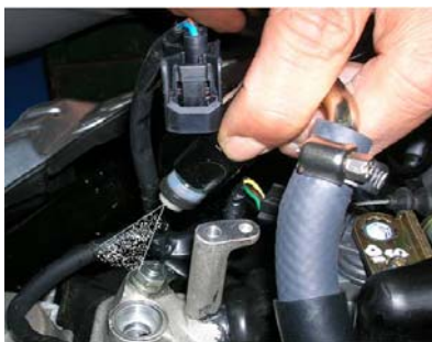
Injection-state atomizing good
