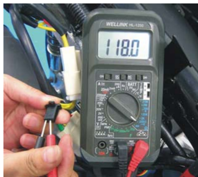
Measurement resistance value
