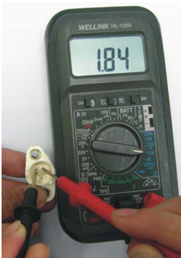
Resistance value measurement
