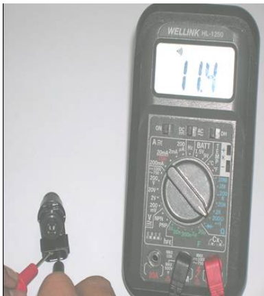
Injector resistance confirmation
