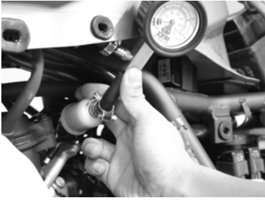
Fuel system pressure measurement
