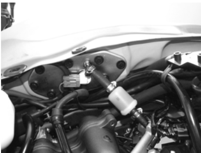
Pressure measurement -fuel pump side
