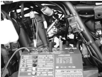
Fuel pump working voltage measurement
