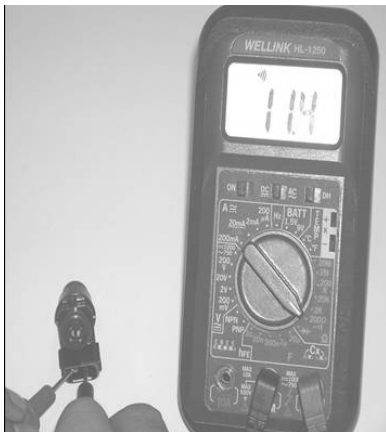
Injector resistance measurement
