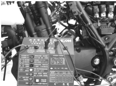
Working voltage measurement
