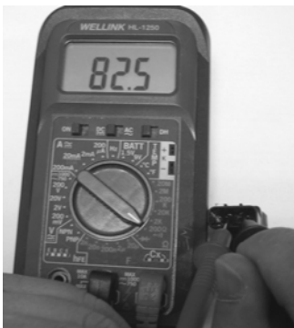
Resistance value measurement of B phase
