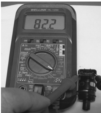
Resistance value measurement of A phase
