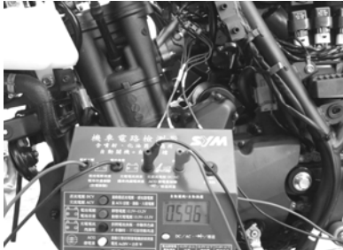
Throttle output signal measurement - close
