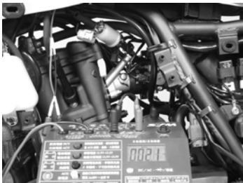
Fuel pump resistance measurement
