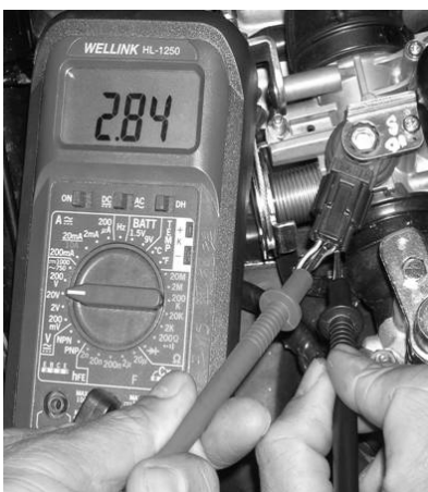
Output voltage measurement
