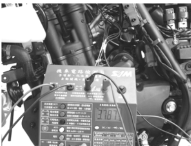
Throttle output signal measurement - full
