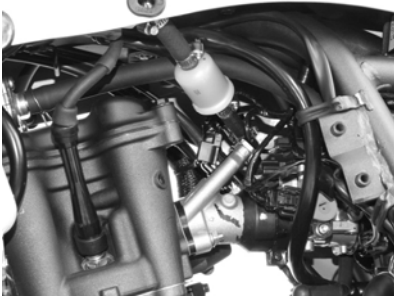
Pressure measurement-injector side
