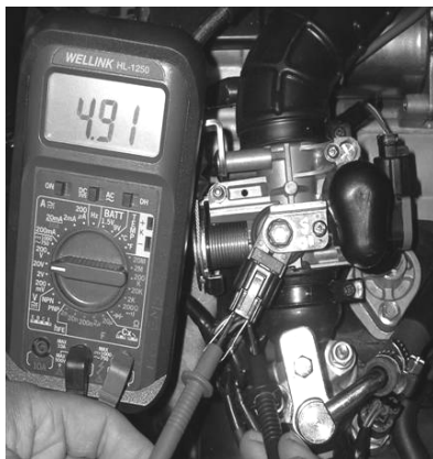
Working voltage measurement
