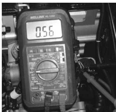
TPS output voltage – throttle fully closed
