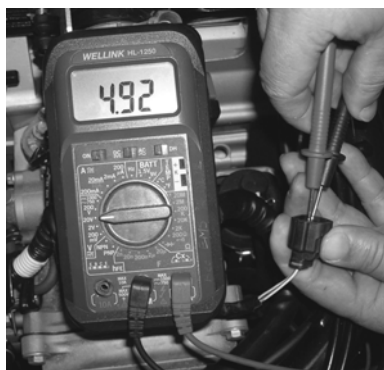
Working voltage measurement
