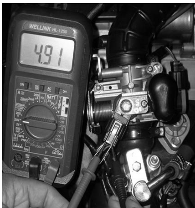
Working voltage measurement
