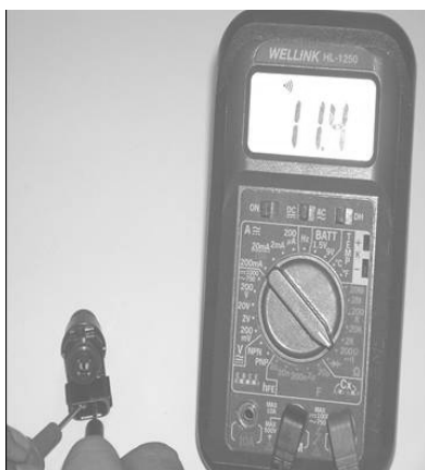
Injector resistance confirmation
