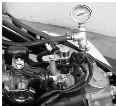
Fuel system pressure measurement
