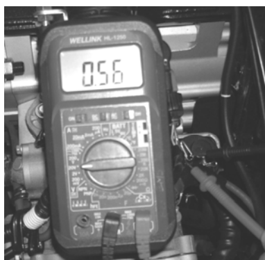
Throttle output signal measurement - full closed
