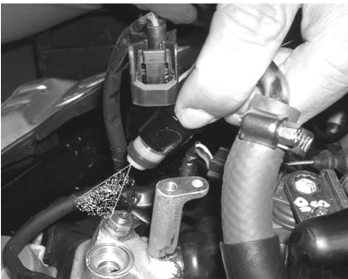
Injection-state atomizing good
