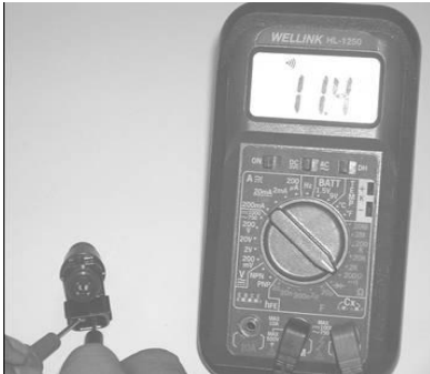
Injector resistance confirmation
