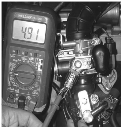
Working voltage measurement
